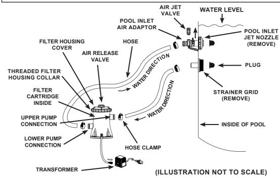
The power cord plug to the 220-240 volt electrical power source of the filter pump must be positioned more than 3.5 m away from the pool walls. Check your local authorities to determine the appropriate standard and requirements for "electrical installation of swimming pools and basins equipment". The following table is for reference only:
